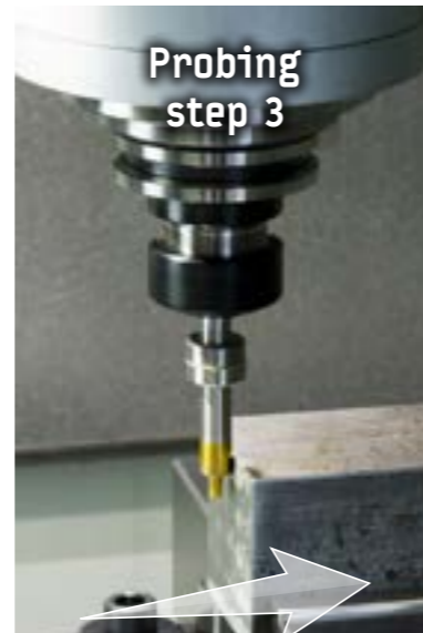
3. When reaching the final position, the edge finder body passes along the edge. Now, the position corresponds to the radius of the tracer.
