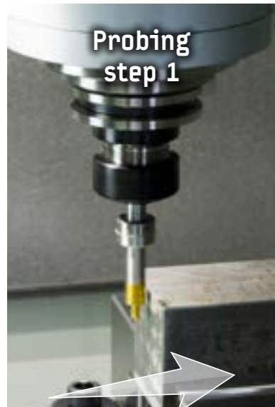
1. The edge finder body can be tilted out from the axis' centre by a gentle tip of the finger and is out-of-the-round.
